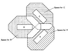
The minimum spacing distance between caravans made of aluminium or other materials with similar fire performance properties should be:
